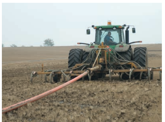
Injection of liquid manure will help to reduce odours and the loss of nutrients such as nitrogen and phosphorus.
