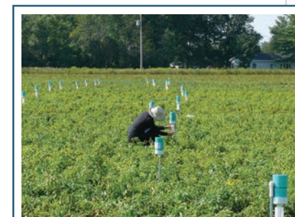
Use rain gauges or catch cans located strategically across the field to measure the actual depth (and volume) of water applied to the crop and the evenness of the application.
