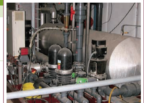
Disinfecting the nutrient solution before reusing will reduce the risk of spreading diseases among crops.
