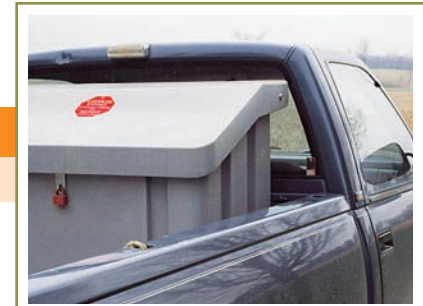
A pesticide storage warning sign must be placed on a vehicle that is transporting more than 500 L of pesticides on any road. The sign must also be displayed on unattended vehicles carrying pesticides.
