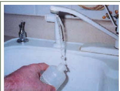
Test the well water once a year for parameters such as nitrate.
