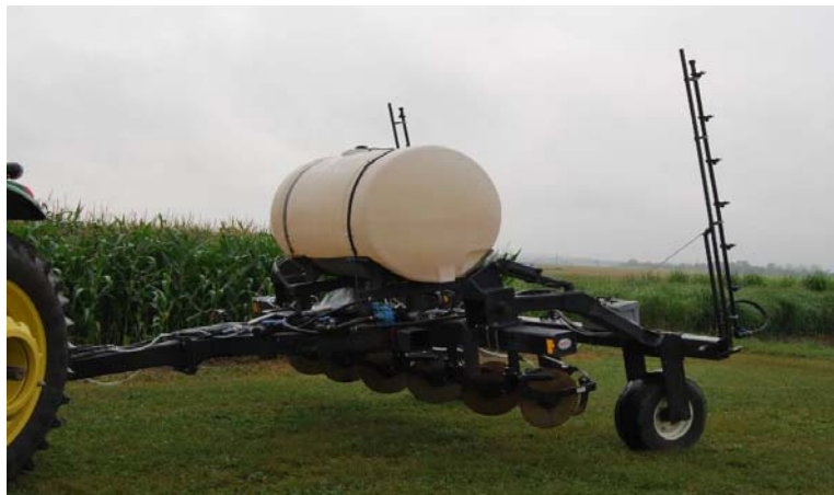
Figure 1. Yetter© Toolbar Applicator Designed For Preplant And Sidedress Nitrogen Applications
