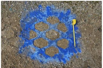
Figure 3. Footprint of 30.5LR32 radial tanker tire at 28 PSI, approx. lug surface area of 1,410cm<sup>2</sup>
