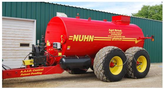
Figure 1. A tanker complete with compressor, airlines and control system for field edge inflation pressure adjustment.
