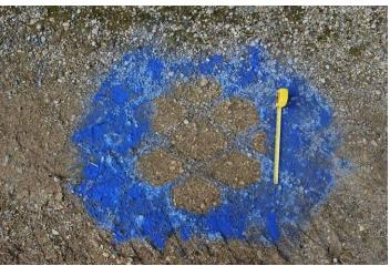
Figure 2. Footprint of 30.5LR32 radial tanker tire at 42 PSI, approx. lug surface area of 1,310cm<sup>2</sup>
