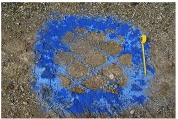
Figure 4. Footprint of 30.5LR32 radial tanker tire at 14 PSI, approx. lug surface area of 2,090cm<sup>2</sup>
